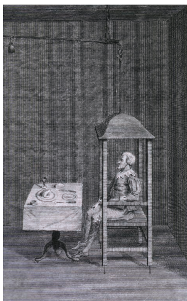
Santorio Sanctorius's balance for tracking the effects of his food intake on his weight.
